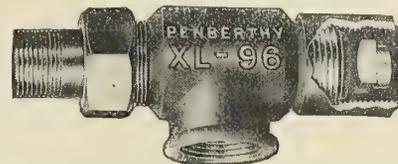
reaching it, as it will work with hot condensation, or it may be located any distance from a steam pump and be worked with water discharged by the sump. When operated with 40 pounds pressure (either steam or water) it will elevate 20 feet, and when operated with higher pressure it will elevate to proportionately greater heights.
